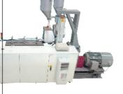
First haul-off machine Haul-off for silicore pipe Widened caterpillar with grooves to fix the silicore pipes
